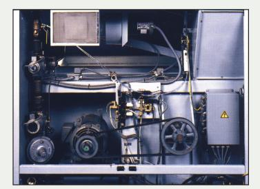
An impressive drying time and finish is achieved by coupling a 25 hp totally enclosed blower motor which moves 13,000 cfm of air with our energy-saving air recirculation system. As soon as a pilot flame is established, the pneumatic air reclaimer goes to work and stays in operation during the entire heating cycle. Our system achieves a 17% rate of hot air reclamation, thereby drastically reducing energy costs.  $( \bullet )$
